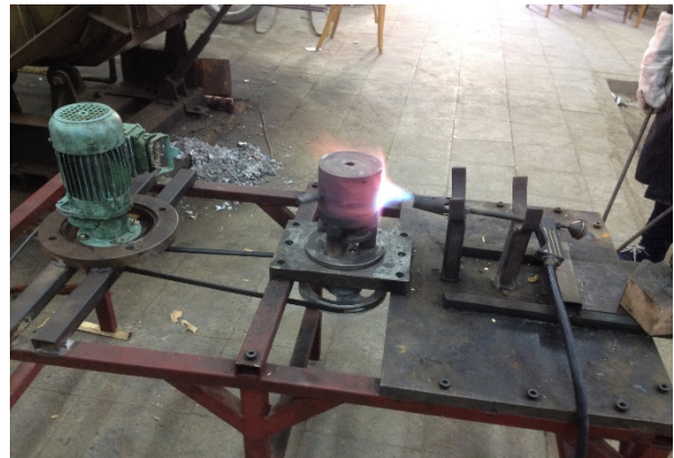
FIG.3. A PHOTO FOR THE VERTICAL CENTRIFUGAL CASTING MACHINE.
